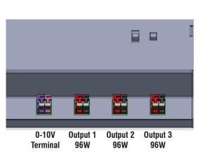
Connect the wiring for the desired output to the appropriate terminals located on the outside of the power supply unit.
