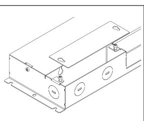
Use a #2 Phillips screwdriver to remove the two (2x) button head screws that are securing the wiring compartment cover, which is the smaller of the two.
