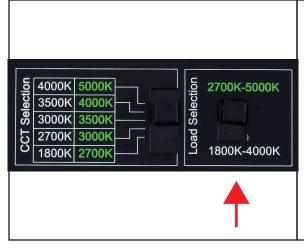
Slide the "Load Selection" switch to the temperature range that corresponds to the unit's connected load type.
