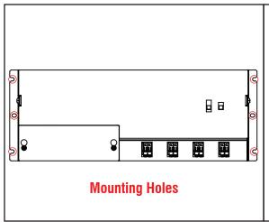
Mount the power supply unit to any indoor surface that is distanced from heat sources and is easily accessible for servicing. The screw holes for mounting are located on each side of the case.
