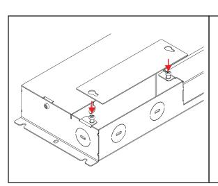
Slide the cover of the wiring compartment back on and retighten the screws with the #2 Phillips screwdriver.
