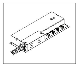
Remove a knockout from the wiring compartment and install the Romex connector with the provided locknut. Insert the Romex cable through the connector, securing it with the integral cable clamp. Splice the black Romex wire to the black wire from the power supply, the white Romex wire to the white wire from the power supply, and the green or bare copper Romex wire to the green wire from the power supply. All connections should be made with wire nuts.
