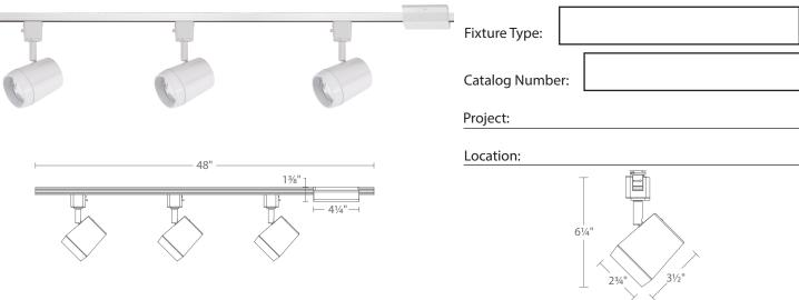
Ideal for residential spaces and lower-mounted commercial installations, the OCULARC 7011-CS combines a high efficacy 5-CCT selectable COB LED with easy-to-use films for three separate beam spreads, along with an
